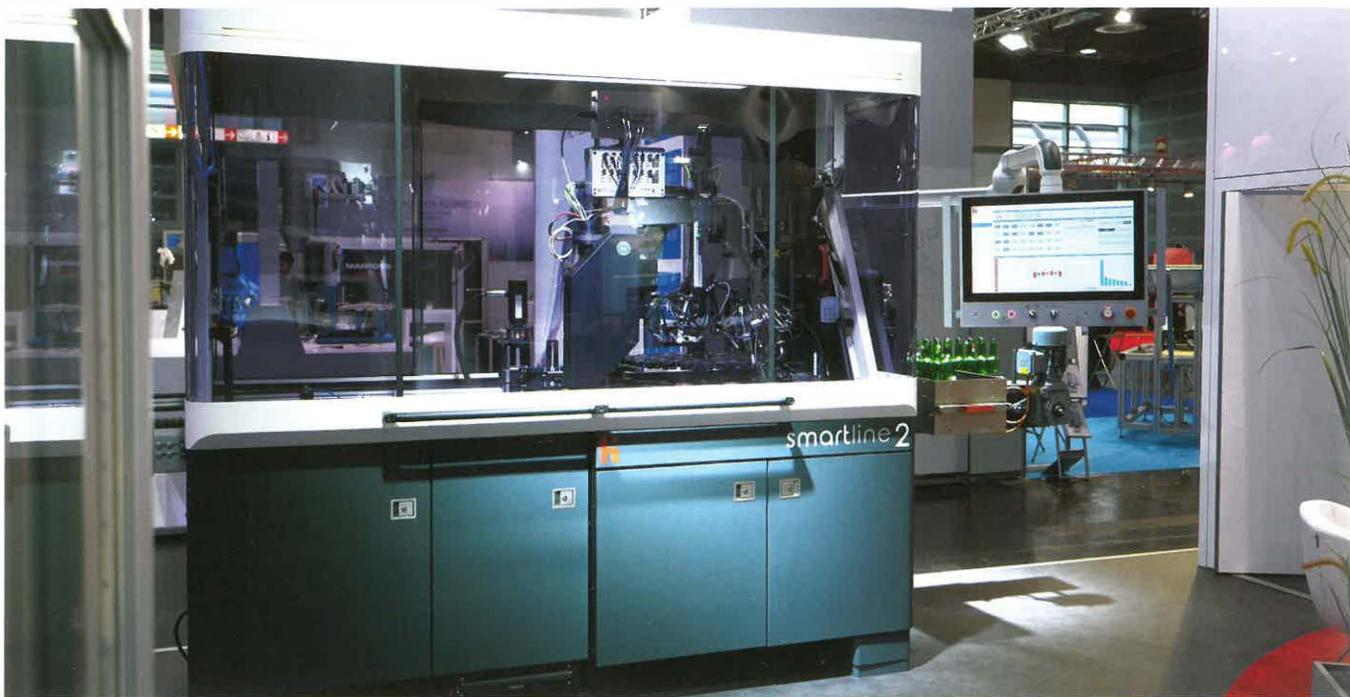
SmartLine 2 is the latest generation of Heye's starwheel inspection machine series.
