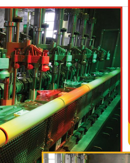
"The latest generation of IS machines can be equipped with sophisticated status lighting to provide enhanced safety, while also increasing mould life expectancy. The status lighting is a coloured RGB-section lighting that colour changes depending on the current status of a section."
