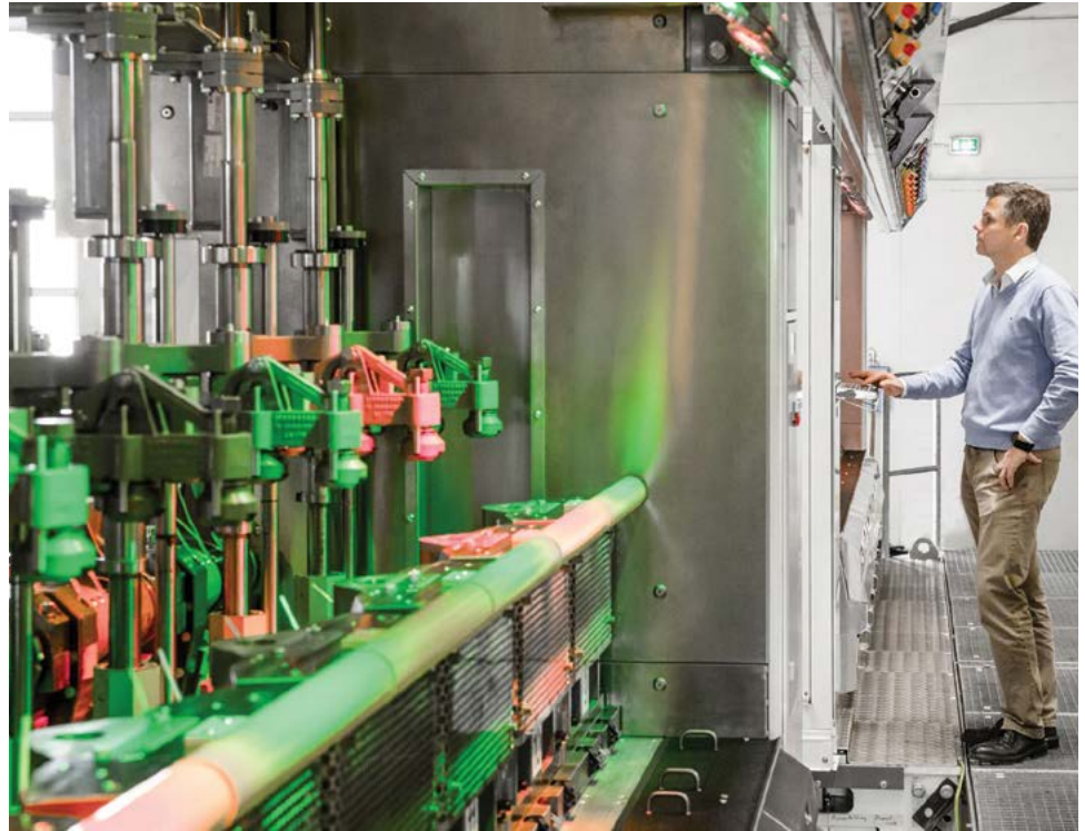
Heye International's coloured RGB status lighting with white lighting option provides enhanced safety, while also increasing mould life expectancy.
