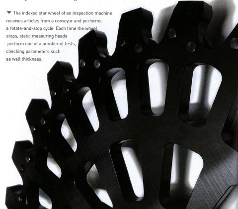
The measurement technology employed in Chrocodile sensors can potentially achieve even higher speeds. The upper limit is set by the container output and transfer mechanisms related to the star wheels.
