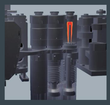
A consistent duration of the plunger within the glass ensures a reproducible wall thickness and therefore high quality.
