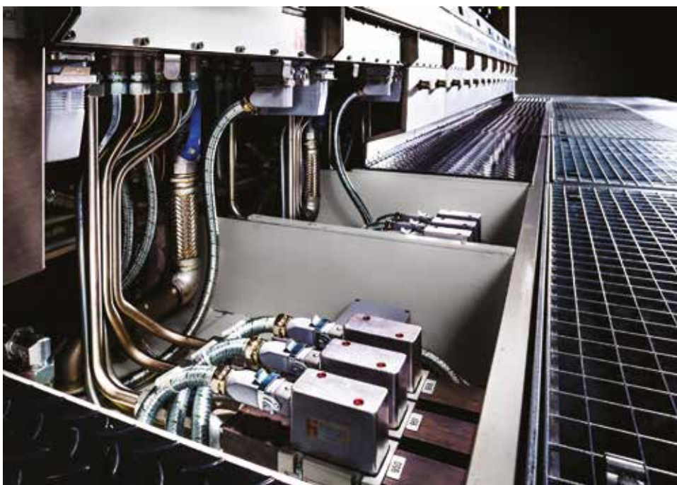
Figure 2: By providing a defined distance between air distributor and box, fixed stainless steel piping is simple to install using proportional valves.
