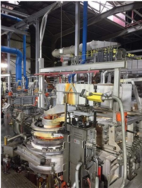
One of the new IS machines is a 12-section 6 1/4in double gob installation, while the second is a 10-section 5in double gob SpeedLine. The production shop's other two lines feature existing Heye IS machines. The feeders for these lines have been modernised with the latest Heye front plates and spout casings.
